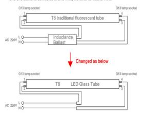
Note: No.1&2 are connected to L wire No.3&4 are connected to N wire (The Inductance Ballast must be removed )
